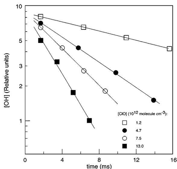
**Figure 2** An example of kinetic runs of OH consumption in reaction with excess ClO ( $T = 296$  K). Experiments were carried out in excess of O<sub>3</sub> in the reactor.
