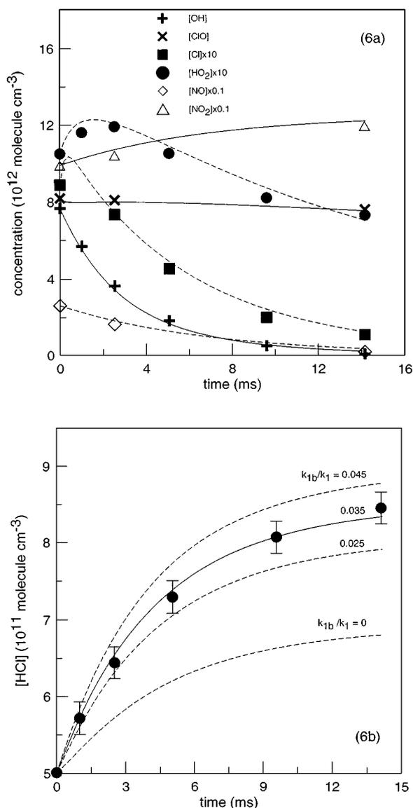
**Figure 6** Example of experimental (points) and simulated (lines) kinetics for the species detected in the chemical system used for the study of the reaction (1b):  $T = 298 \text{ K}$ ,  $[\text{O}_3] = 3.7 \times 10^{14} \text{ molecule cm}^{-3}$ .
