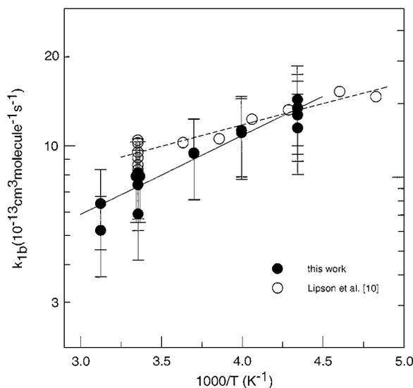
**Figure 8** Temperature dependence of the rate constant for the HCl + O<sub>2</sub> forming channel of reaction (1). The errors shown for the data from the present study represent conservative 30% uncertainty; the uncertainties on the individual data points were not quoted in Ref. [10].
